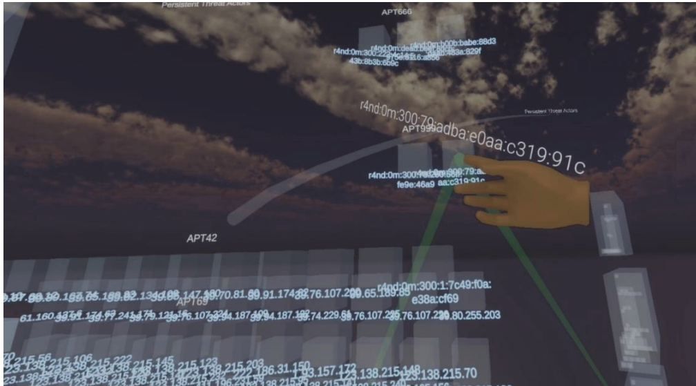
Figure 12: The user can select nodes either (1) from afar, with a pointer or (2) by touching them with their virtual index finger (rendered based on inputs from a VR controller). The selected node’s name (in this case, the IP address) is displayed next to the VR hand. The node’s incoming and outgoing edges are kept visible while other edges are disabled.
