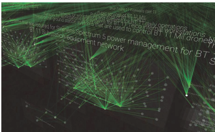
Figure 5: VDE 3D display of network topology and traffic focusing on a single Blue Team network topology (“Zoom” on “Details-on-Demand”, per (Shneiderman, 1996)). Additional videos of VDE can be found: https://coda.ee/vde
